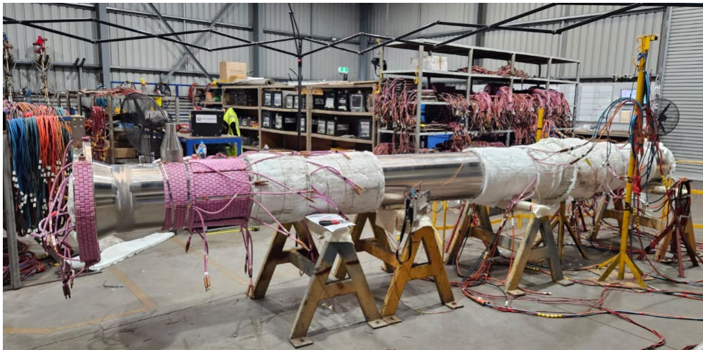
Reactor successfully heat-treated and preparing for machining and final assembly
