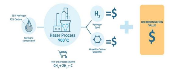
The Hazer Process® aims to replace the currently utilised hydrogen manufacturing methods, such as 'steam methane reforming', which necessitates high CO<sub>2</sub> emissions and expensive CCS (Carbon Capture and Storage) to address these emissions. Another hydrogen-producing method using electrolysis is highly energy and cost intensive and requires substantial water and renewable energy.
